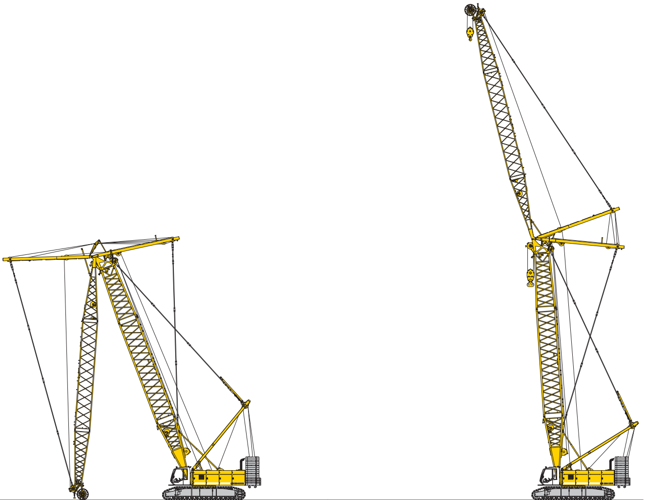
Erecting of main boom and luffing jib
