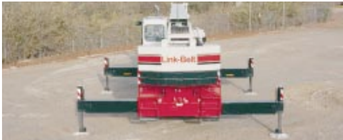
Fully Extended Outriggers 20' 6" (6.25 m) Spread
