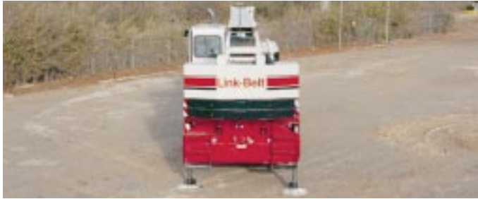
Retracted Outriggers 7' 9" (2.36 m) Spread
