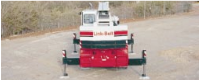
Intermediate Outriggers 14' 2" (4.32 m) Spread
