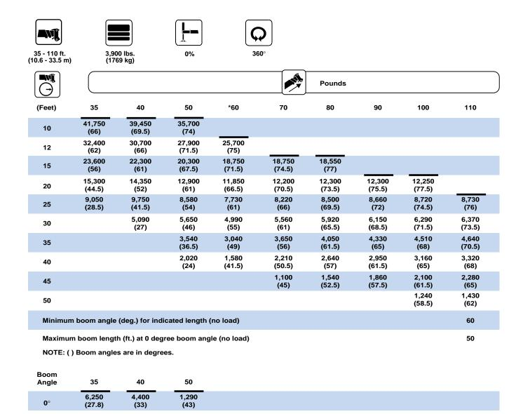
\*60 ft. boom length is with inner-mid extended and outer-mid & fly retracted.
